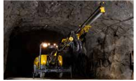
Boomer S1 can cover a large work area thanks to 70 meters of water hose and extended electrical cable.
